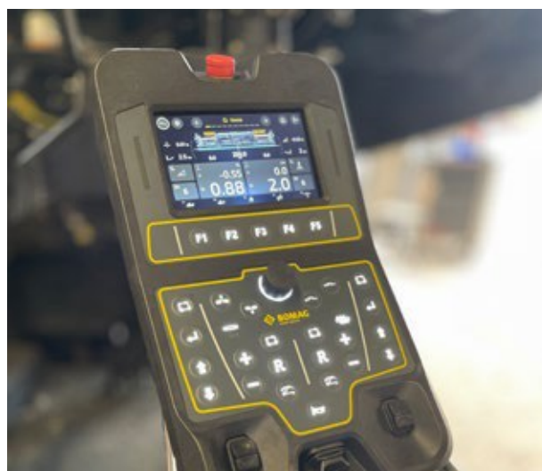
Screed side panel with large full graphic display - direct access to all major functions
